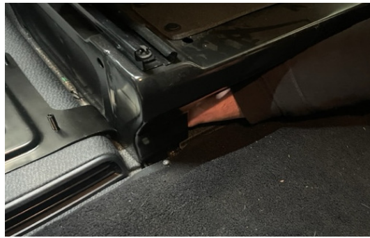
Use black screw 2x to mount bracket DO NOT TIGHTEN YET
