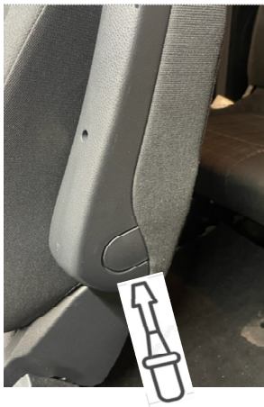
Flip out the cover from armrest remove armrest from seat cover up with special cover and tighten with screw
