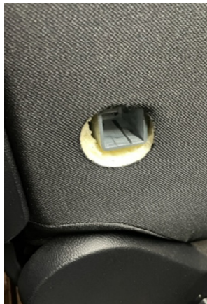
Flip out the cover from armrest remove armrest from seat cover up with special cover and tighten with screw
