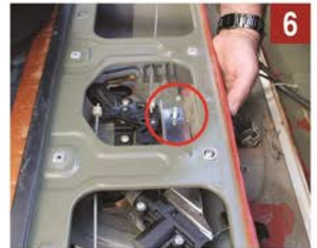
6 Fasten up the screw like in the picture (From below to above)
