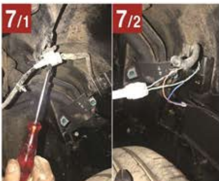
7/1 7/2 You can cut off the power by removing left-rear mud guards
