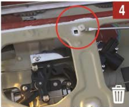
4 Remove the clips like in the picture
