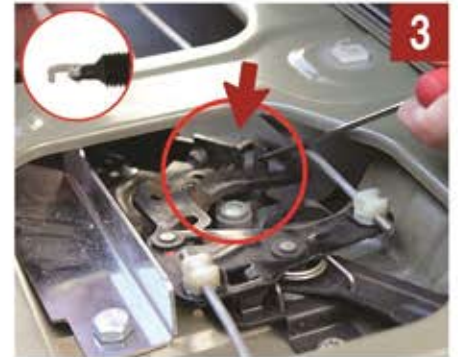
3 Mount the kit at the end of the mechanism to the triangle piece
